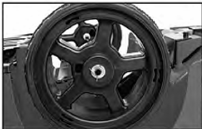
4. Insert gaskets, lock with bayonet locks.
