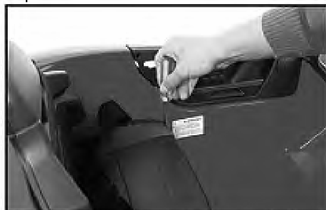
10. Tighten the screws on the seat.
