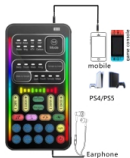
Mobile Phone Connection Diagram with Round Hole Headphone Jack
