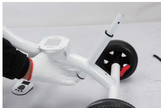
11.Pass the steering shaft through the steering tube
