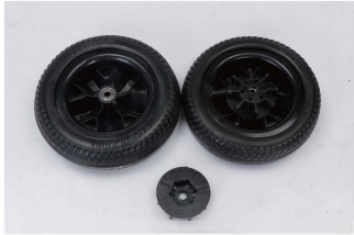
4.Attach brake discs to both rearwheels
