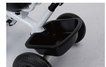
24.Install the back basket and tighten the screws to fix it
