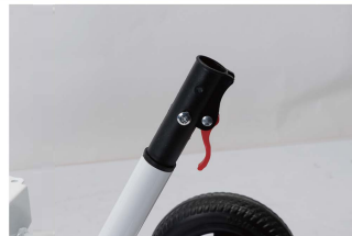
12.Install the quick release interface, and wait for the bean to pop out of the hole
