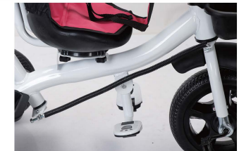
27.Steering wire installation effect
