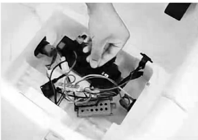
5. Install the power supply: Connect the power cord according to the positive and negative poles. The red terminal connects the red connector. Black terminals are connected to the black connectors.
