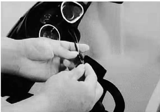
3. Music Plug-in Connection. Connect the lines before installing the steering wheel.
