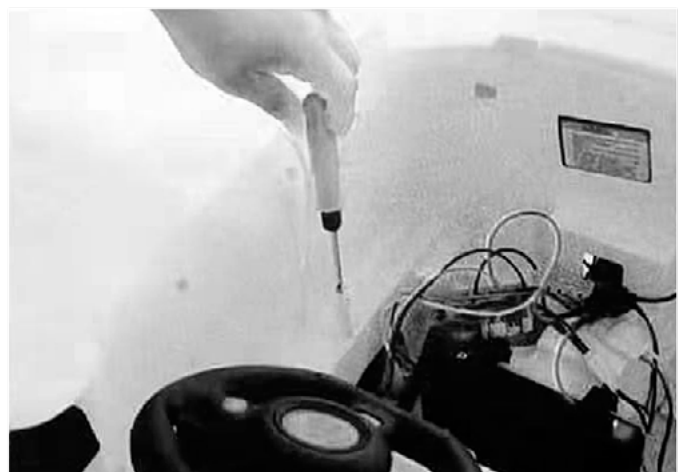
6. Seat Installation: Remove the body screw.
