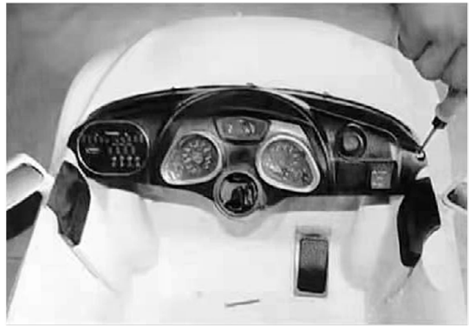
2. The instrument panel passes through the steering wheel shaft, and the left and right screws are fixed.
