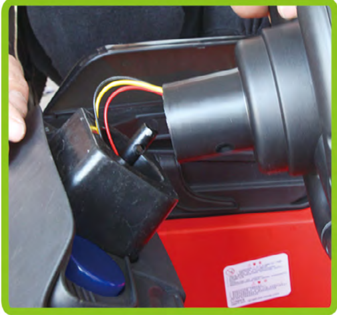
9. Put the handlebars in place on the axle, taking care of the cables!
